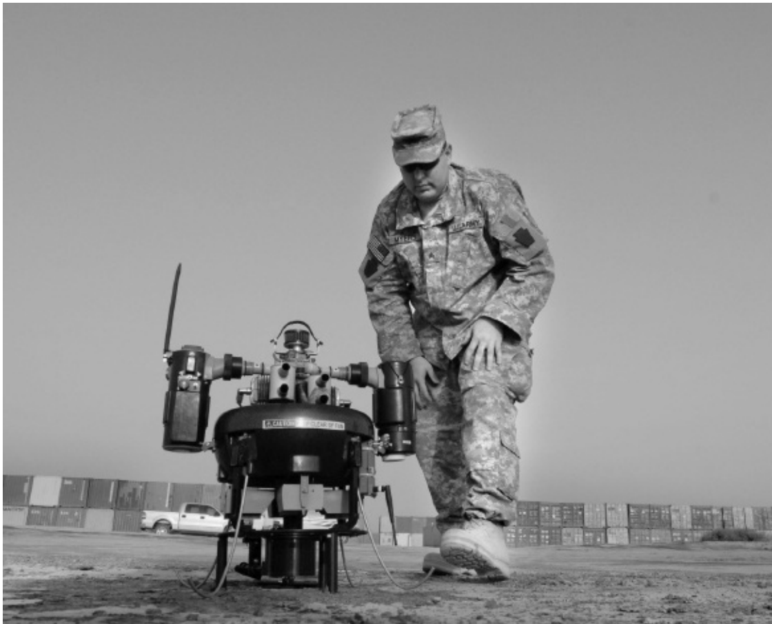
A micro air vehicle (MAV) prepares for its first combat mission in Iraq, in 2005. Many of DARPA's advanced MAV's are now small enough to fit in the palm of the hand. (U.S. Department of Defense, photo by Sgt. Doug Roles)
