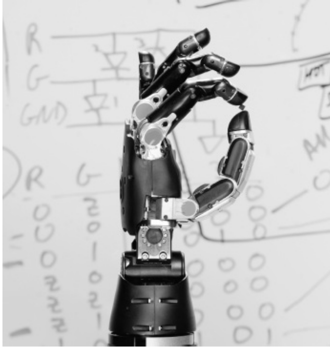
The DARPA Modular Prosthetic Limb. The work advances robotics but is it helping warfighters who lost limbs? (U.S. Department of Defense, courtesy of Johns Hopkins University Applied Physics Laboratory)
