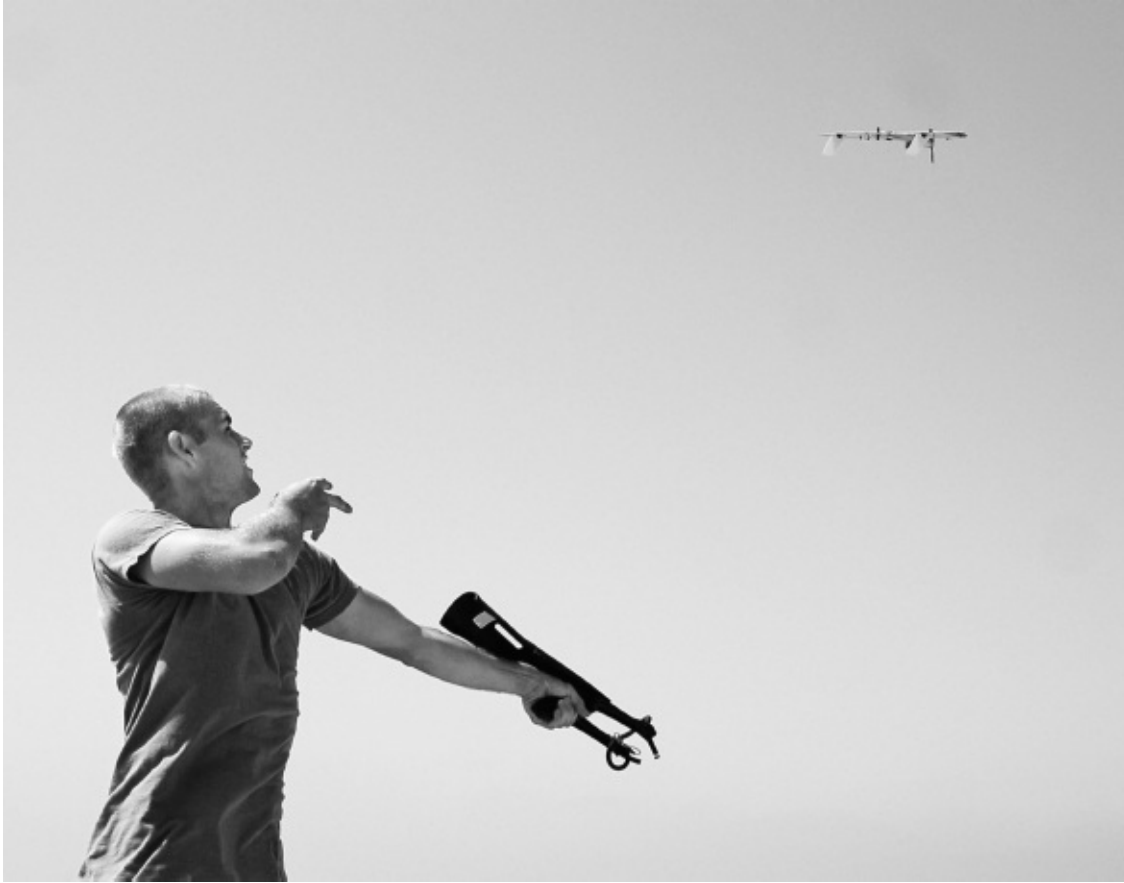
The seven-ounce Wasp drone, part of DARPA's Combat Zones That See, gathers real-time video and works in a swarm. (U.S. Department of Defense)
